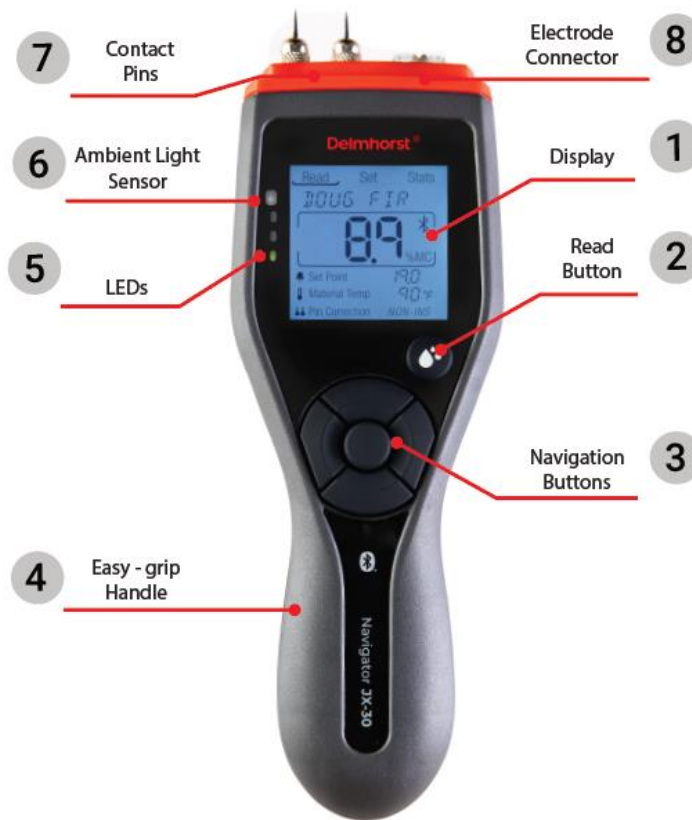
Figure 1: Meter components
