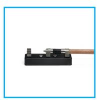
Moisture content standard used to verify moisture meter calibration. Has electrical resistance values of 16% and 22% to test against.
